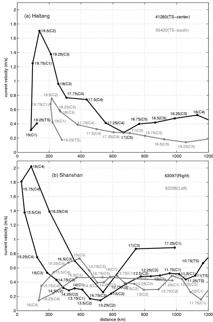
Fig. 6. Current speed of drifters under the influence of (a) Hai-Tang and (b) Shan-Shan in chronological order versus the distance from drifter to storm center. Storm intensity (Saffir-Simpson Scale) and indicated time (in month day) are also marked.
